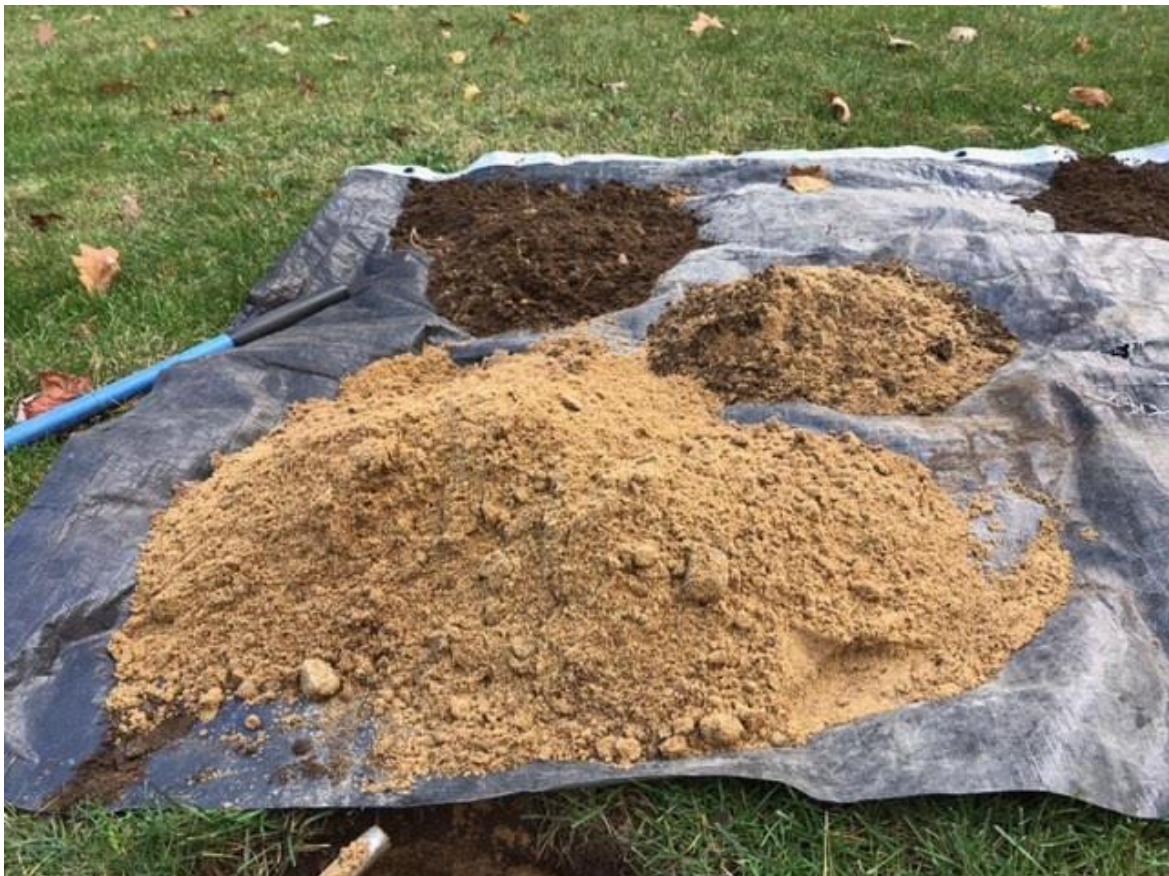
FIELD E – Observation hole #1 sand and stone
