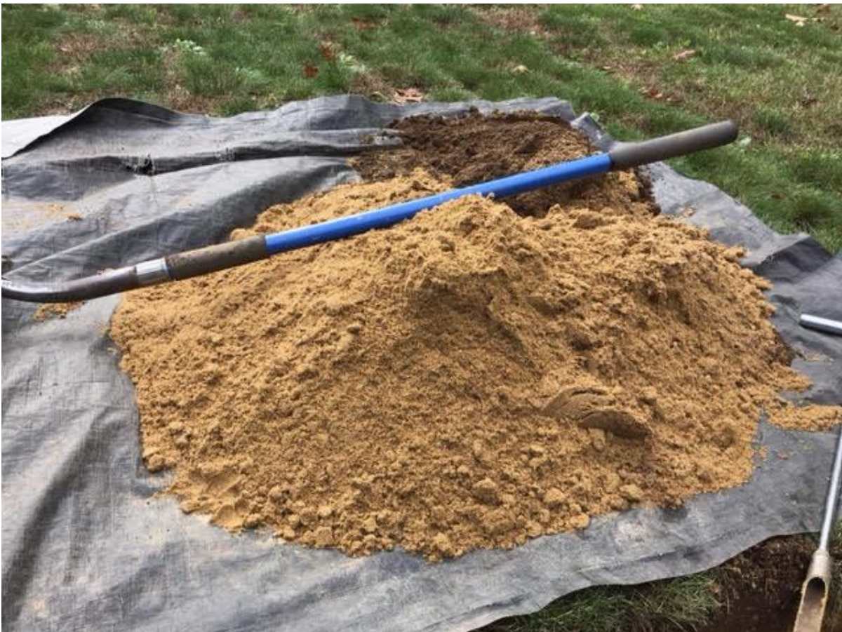
FIELD E - Observation hole #3 sand and stone
