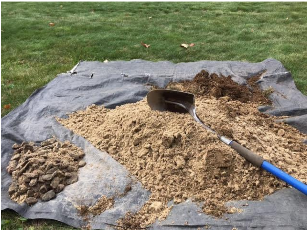
FIELD D – Observation hole #8 sand and stone
