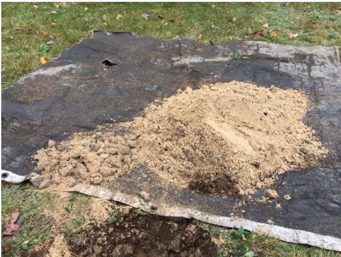
FIELD C – Observation hole #1 sand and stone
