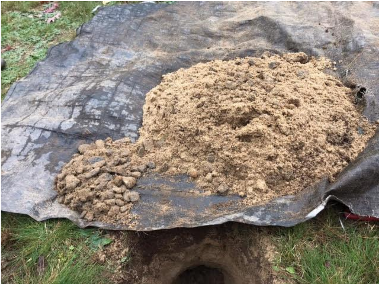
FIELD C - Observation hole #3 sand and stone
