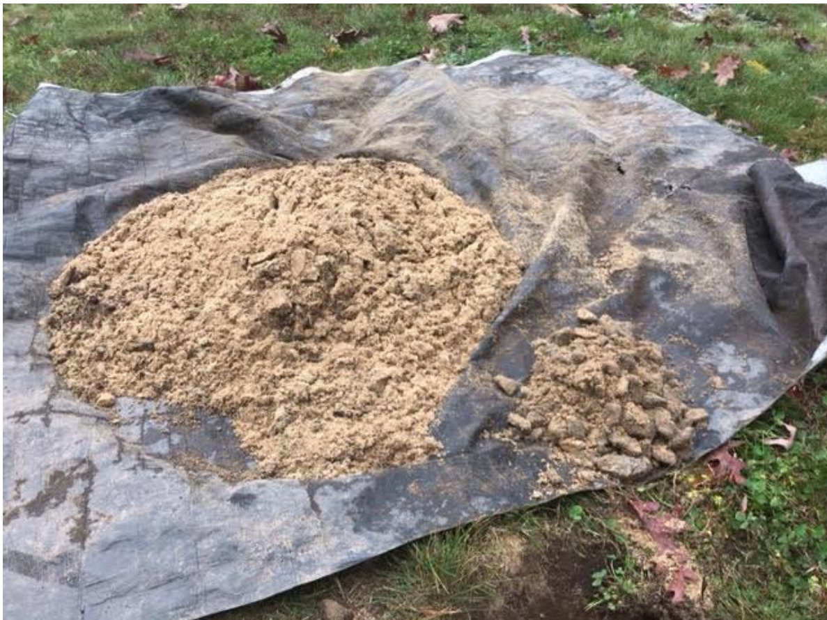
FIELD C – Observation hole #4 sand and stone
